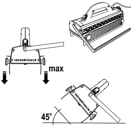
For best results, the protective plates need to always be fully extended and the reason is that at this distance the Infra Red Rays will penetrate deeper in to the material and as a result, more effective without burning the wood. Make sure that the working area is well ventilated. Old paint discards could be toxic, make sure to collect the paint remains and throw away in the right disposal at a waste station.
