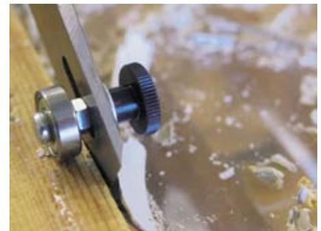
Remove putty with "Chisel with Roller". The tool Chisel with roller is a simple tool to use and does not put any pressure on the glass. Be careful not to hit the nail on the glass to hard.
